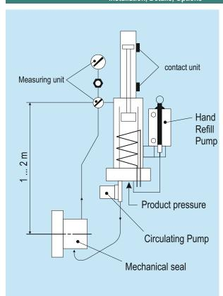
Operating and installation diagram for a PBS system. The PBS pressure booster must always be installed higher than the mechanical seal. The barrier fluid flows via the return pipe into the vessel and is cooled. The exchange of fluid takes place by the thermosiphon principle or by forced circulation, e.g. with a pumping screw. Connection pipes to the seal should be designed with as little resistance as possible.
