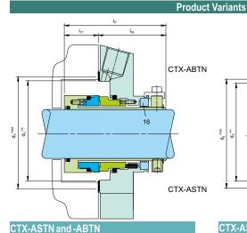
Single seal for operation with unpressurized quench for standard (S) and big bore (B) seal chambers. Same as CTX-ASPN and -ABPN but with throttle ring (item 16). The cover has auxiliary connections for flushing and quench. Throttle ring: PTFE carbongraphite reinforced (T12).
